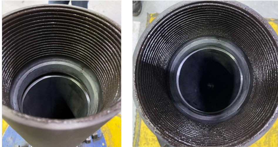
Figure 1: Thread Compound Application
