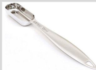
Figure 1: Example of Dope Application Metering Tool (DAMT)
