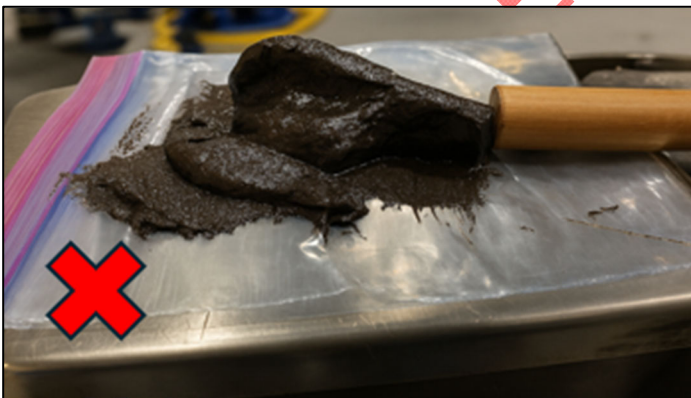
Figure 3: Examples of Excessive Dope Amounts
