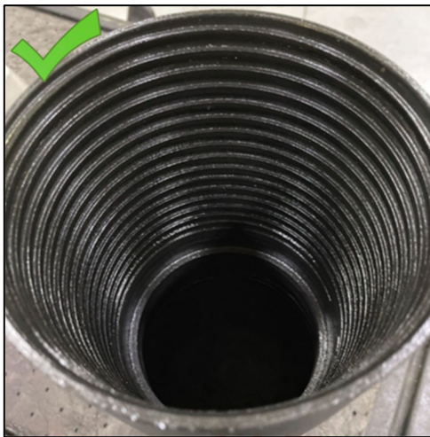
Figure 2: Example of 6.0" OD Proper Dope Amounts and Application
