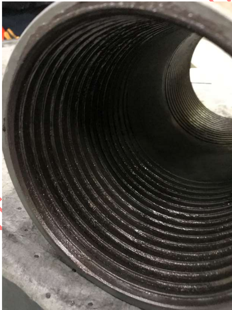
Figure 1: Proper Thread Compound Application
