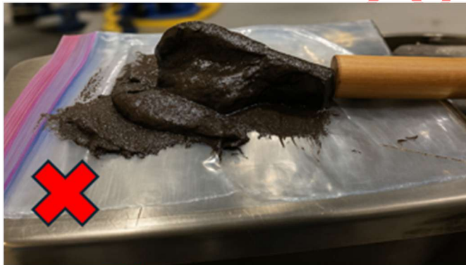
Figure 2: Examples of Rejectable Dope Amounts
