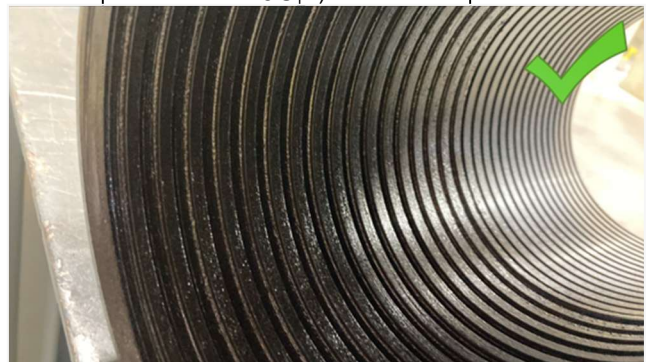
Figure 3: Example of proper dope application
