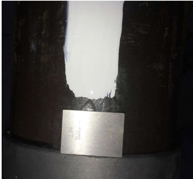
Figure 2: Acceptable Make-up Position for USS-TALON HTQ®
