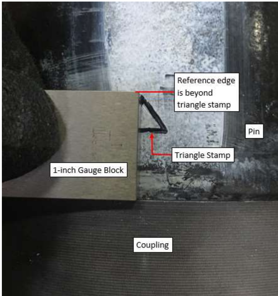
Figure 3: Unacceptable Make-up Position USS-TALON HTQ®
