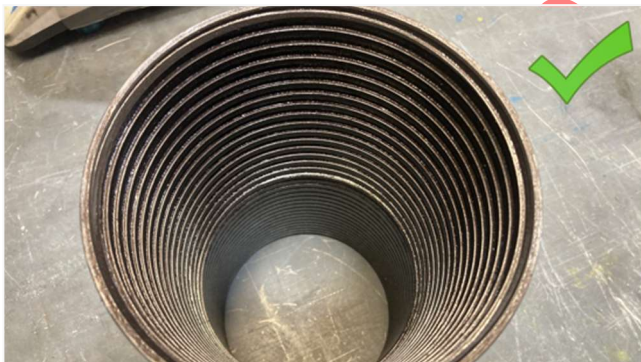
Figure 3: Example of proper dope application
