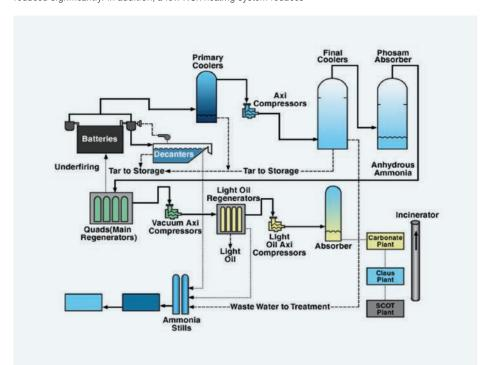
Figure 16. Clairton Plant By-Products Process Flow Diagram.
