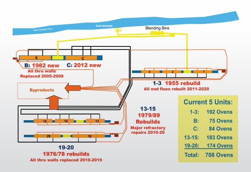
Figure 7. Clairton Plant – Battery Configuration in 2019.
