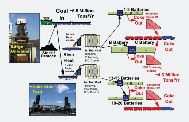
Figure 4. Clairton Plant – General Plant Process Flow Diagram: showing from left to right; the coal being brought by barge to the plant, coal blending & pulverizing operations, coal being charged to the batteries, and coke produced, screened, and loaded into railcars for customer delivery.
