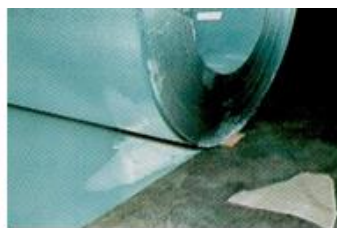
Figure 2. White rust on the surface and sidewall of a galvanized coil.
