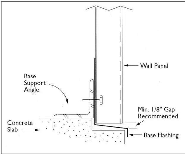
Figure 19. Schematic of proper siding installation.
