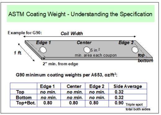
Figure 1. Understanding the ASTM triple-spot, single -spot specifications
