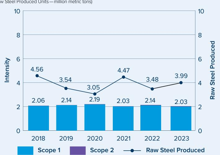
The GHG emissions intensity is based on the total quantity in metric tons of GHG emissions calculated in accordance with GHG Protocol and EU ETS standards divided by the total quantity in metric tons of raw steel produced in the EU as published in the U. S. Steel Annual Report and that is processed into finished steel products.
