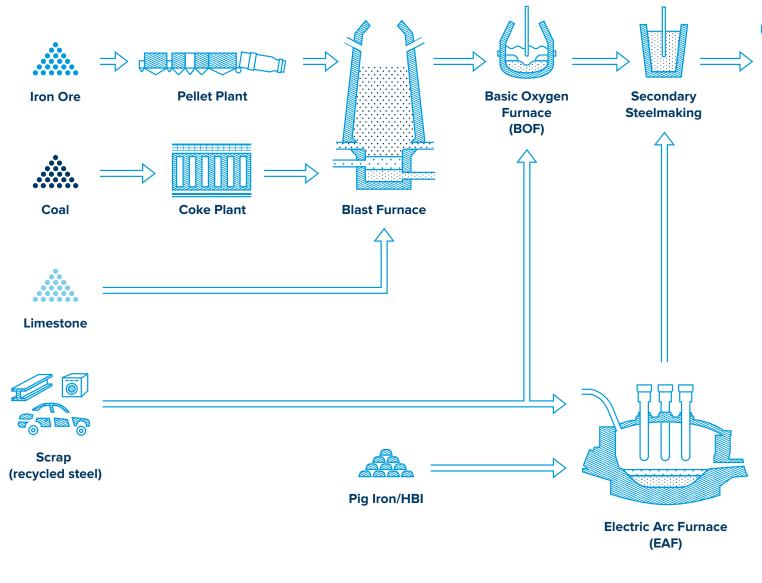
Integrated steel mill (BOF) vs mini mill (EAF) process and equipment requirements
