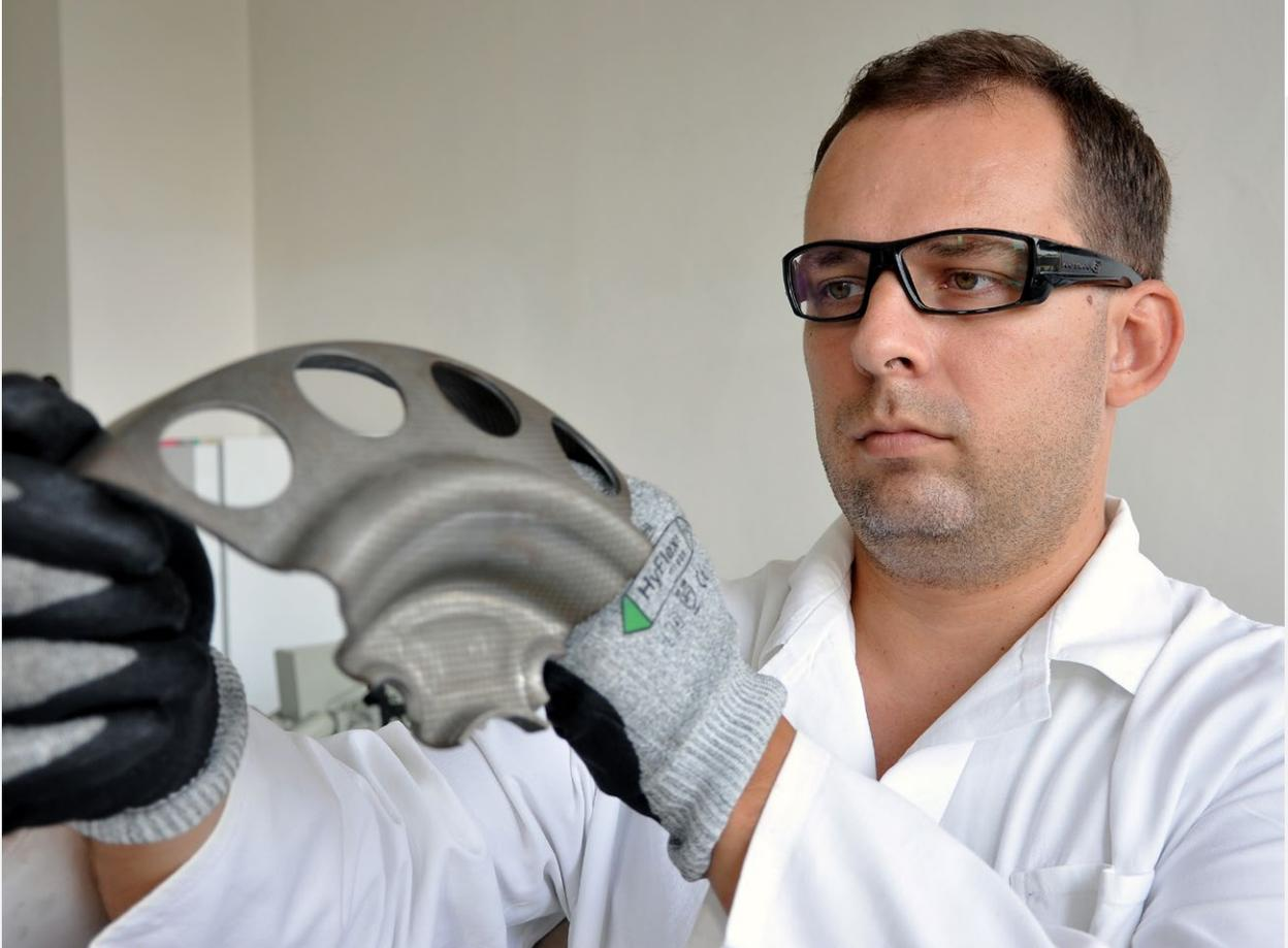
strength steels (AHSS) with increased strength and formability for the automotive industry. This has allowed new AHSS dual phase (DP) highly formable (HF) grades with an ultimate tensile strength of 800 MPa (DP800HF and DP1000) to be added to the USSK product portfolio. In addition, through the innovative application of new technology, USSK has expanded its product mix to include thinner and wider coils.
