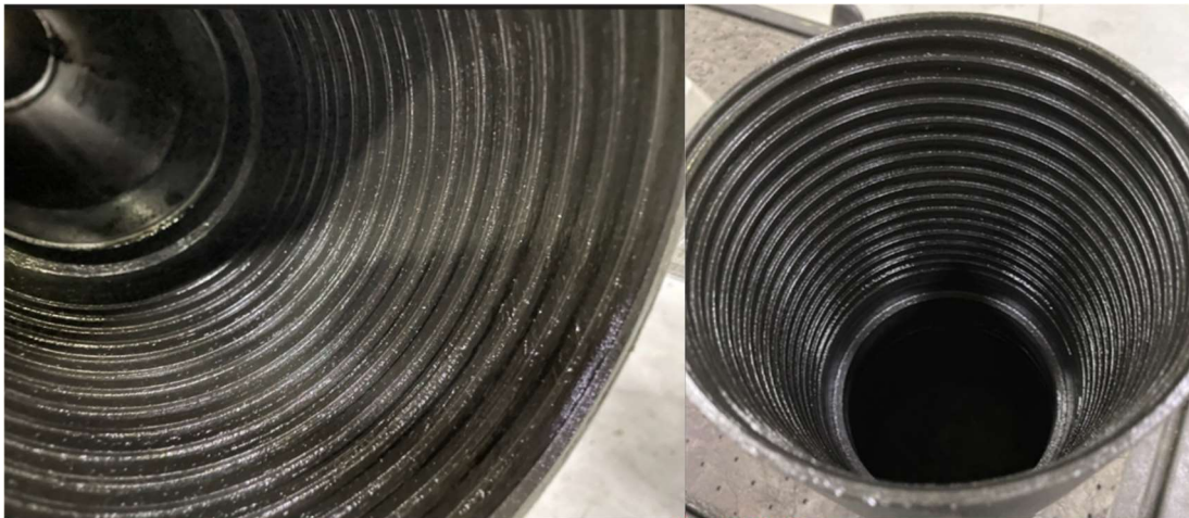
Figure 1: Proper Thread Compound Application
