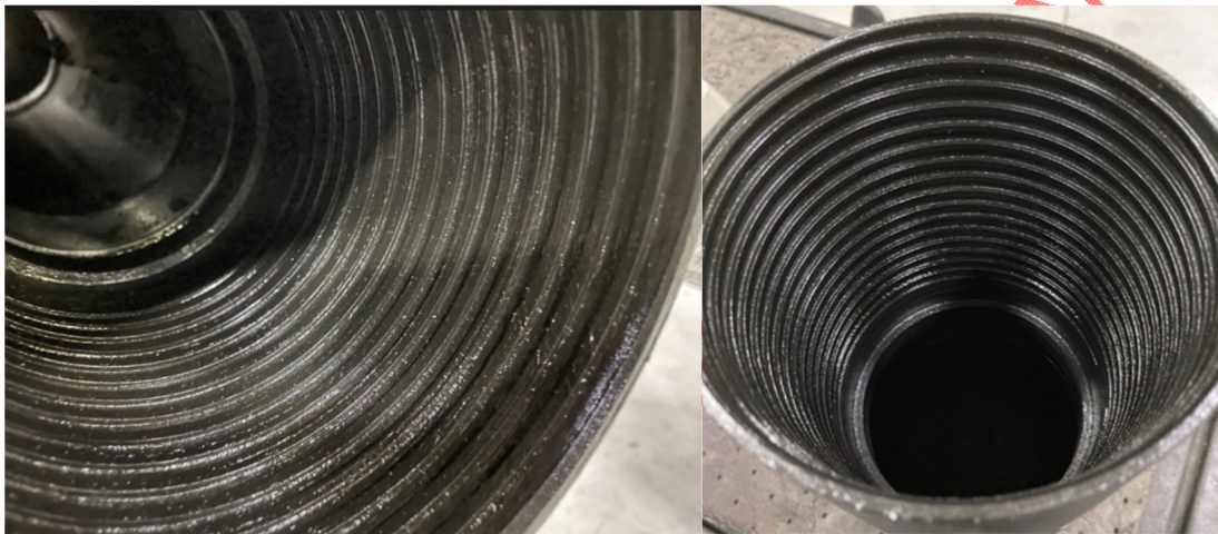
Figure 1: Proper Thread Compound Application
