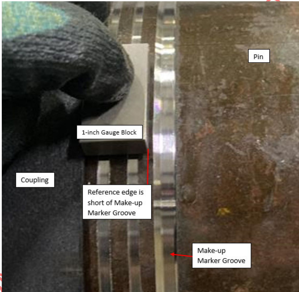
Figure 6: Unacceptable Make-up Position USS-TALON SFC™
