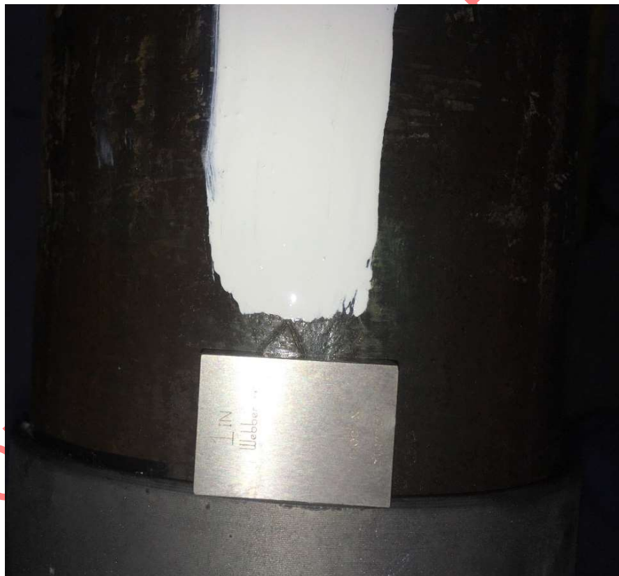
Figure 2: Acceptable Make-up Position USS-TALON HTQ®
