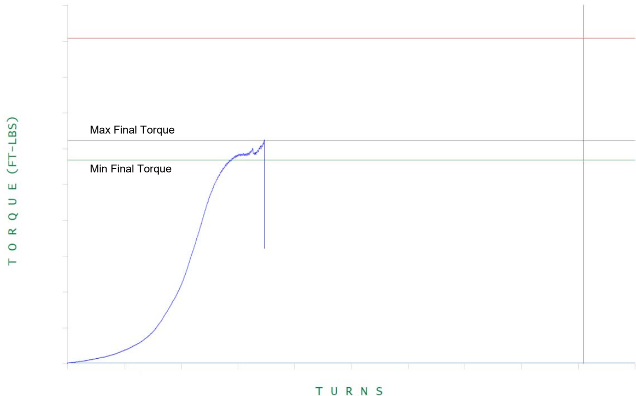
Figure 10: Yielding/deformation prior to final torque (Connection shall be rejected)
