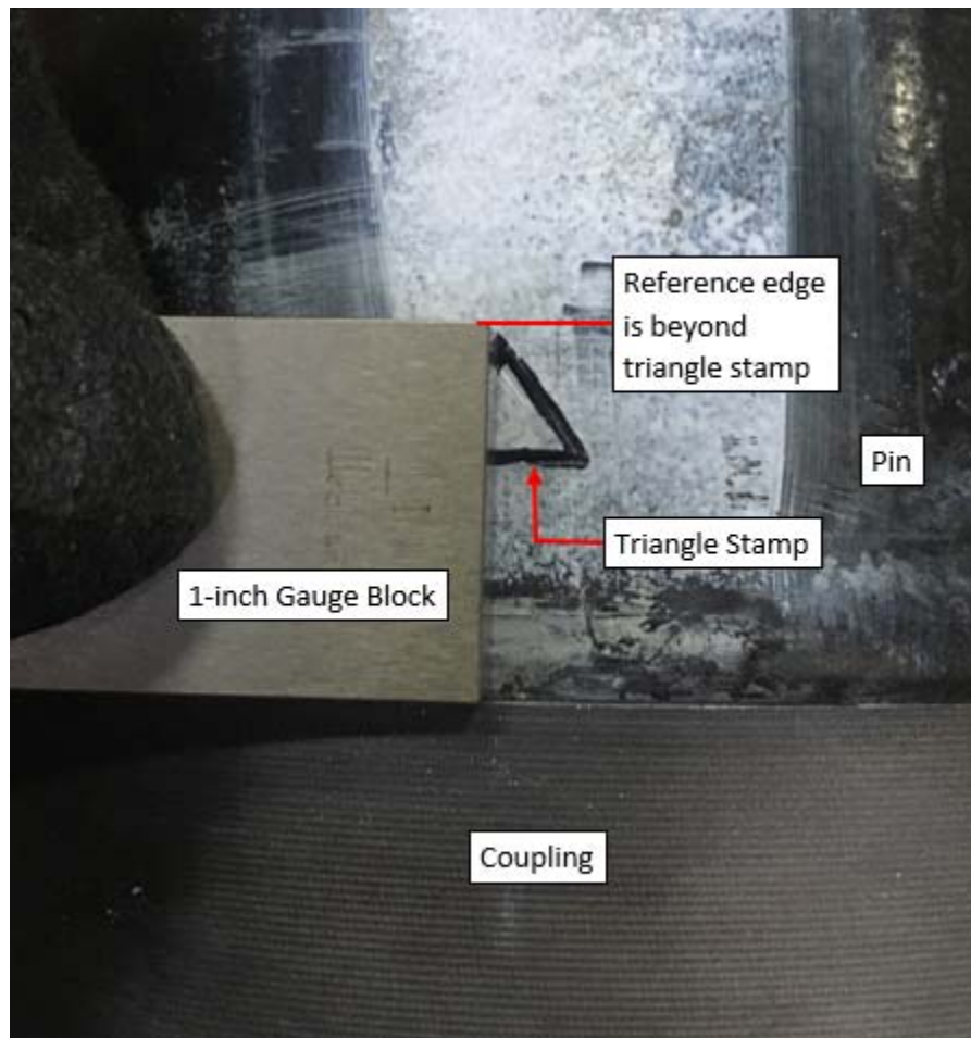
Figure 3: Unacceptable Make-up Position USS-TALON HTQ™
