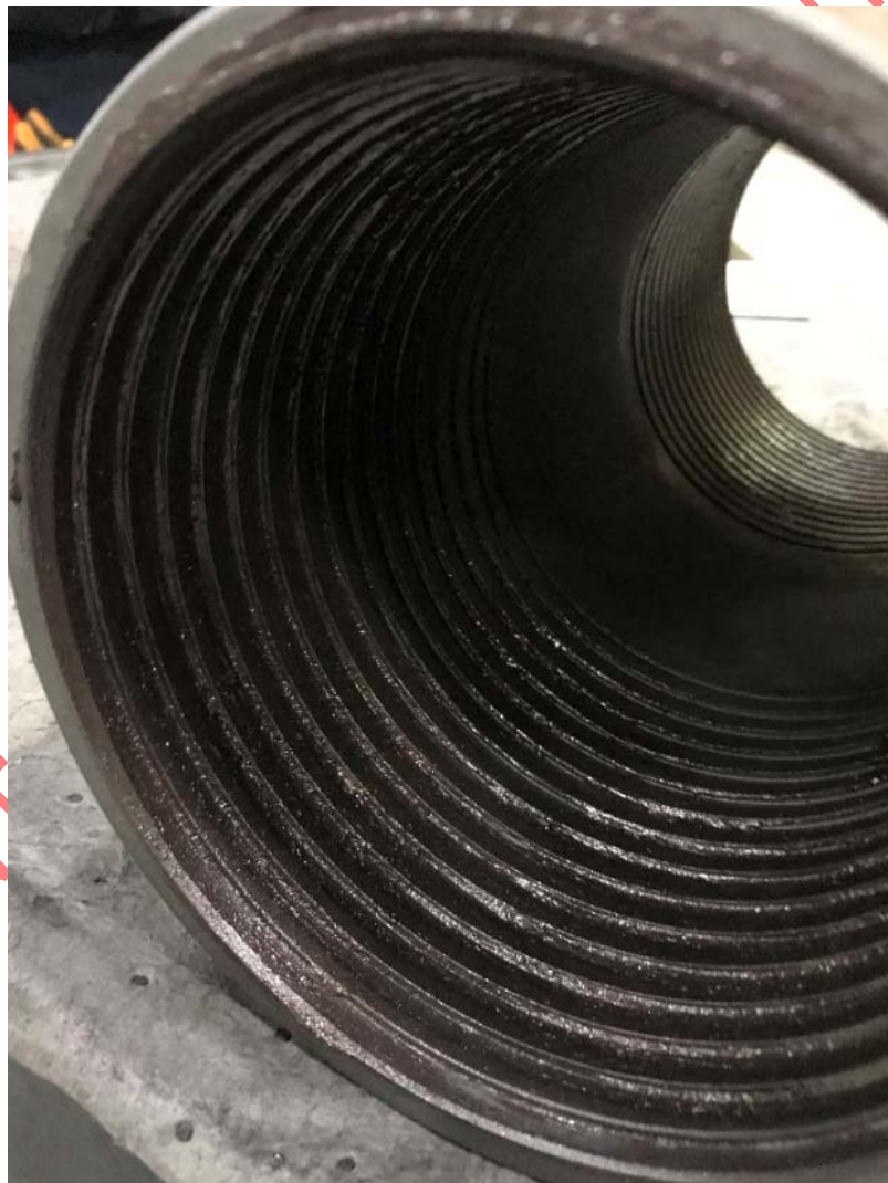
Figure 1: Proper Thread Compound Application
