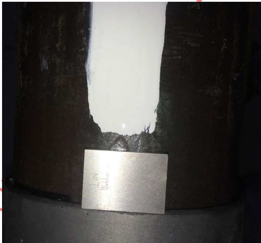
Figure 2: Acceptable Make-up Position USS-TALON HTQ™
