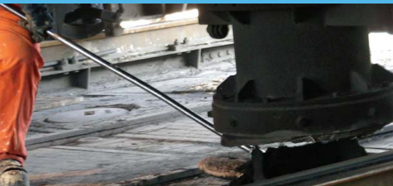
Figure 8. Lidman replaces the lid after the coal has been charged into the battery
